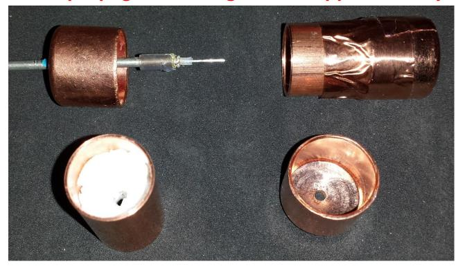
Tube dimensions: 1.02mm thick, 14.34mm ID, 15.85mm OD, 28.89mm long
